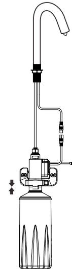
Fill with liquid soap and clip soap container into the pump and controller unit.
