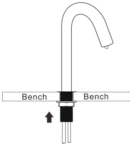
Place hose and control cable through bench top, then tighten nut to secure soap dispenser (Careful not to over tighten and damage bench top)
