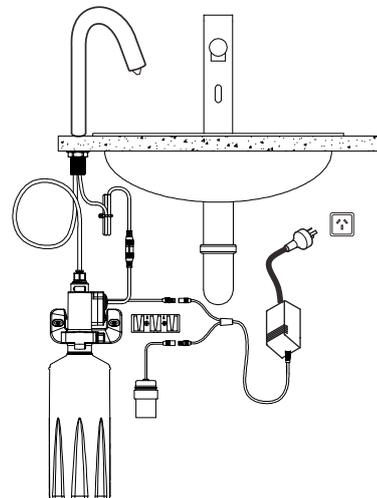
If AC/DC with battery back up, plug battery box into transformer and then plug in to mains socket.
