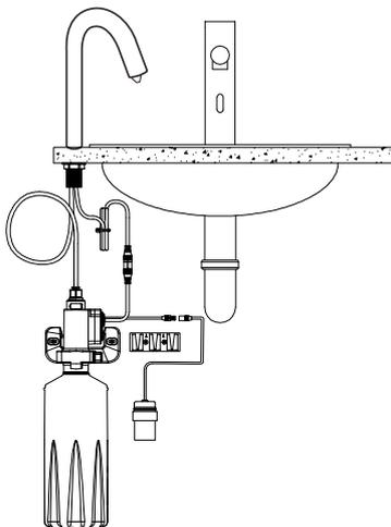
If battery only, plug battery box into power cable.
