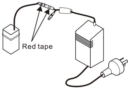
2. Connect transformer (battery box if DC only) to face plate.
