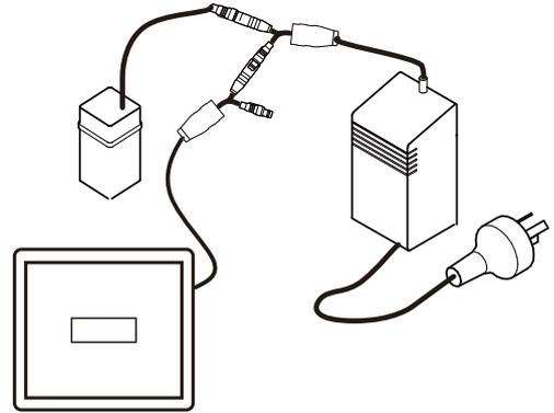
3. Connect solenoid valve to face plate plug.
