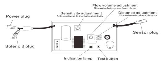
**Sensitivity** – this makes an adjustment to the sensitivity of the sensor. Effectiveness of sensor can be compromised if too much silicone is used on install or the sensor is not installed in the correct area. Increasing the sensitivity and/or sensor distance may help.
