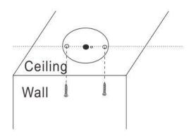
For Twin/Trough urinals – ensure sensor plate screws are aligned facing the wall:
