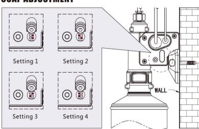
To adjust flow settings, lift cover next to button on pump control and using a small screwdriver, carefully move white switches to the desired setting. Setting 1 is the highest and Setting 4 the lowest. Setting 4 = 2mls.
